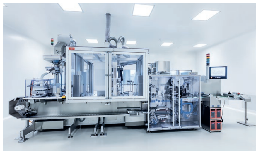
The innovative desiccant blister is packaged on an appropriately modified Blister machine B 1240 from Uhlmann.
